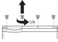
Rotate the door handles as per the diagram and move each to the other door.
